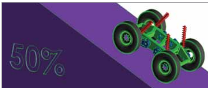
Motor selection simulation - inclined slope with “gravel like” traction
